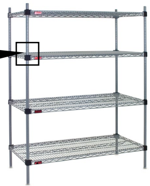
channel of shelf corner fits into slot of collar attached to split sleeve
