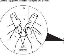
Note: If using aluminum split sleeves, set aside retaining rings until later.
