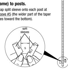
Step 2 - Assemble 4-sided truss frame to posts.
