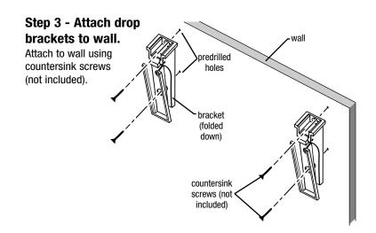
\* **IMPORTANT**: Wall mounted units must be attached to a properly constructed and sound wall. For walls constructed of wood or steel studs, the mounting points must be directly on the stud or suitable in-wall-grounds of plywood or sheet metal. Eagle Group cannot be held responsible for the failure of the device or any other devices due to improper installation.
