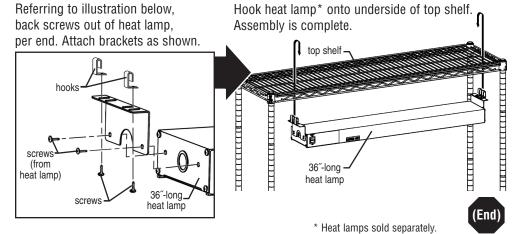
Display unit accommodates packaged heat lamps\* up to
