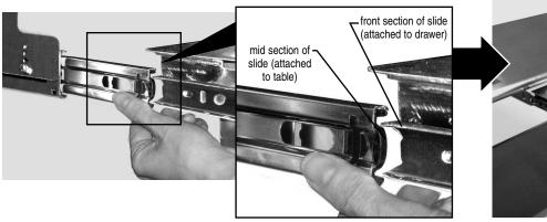
Carefully align front slide section (attached to drawer bowl) with mid slide section (mounted to table), and close drawer fully. Some resistance is normal as you reassemble drawer slides.
