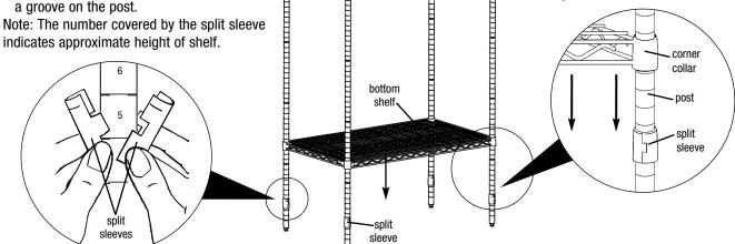
Note: If using aluminum split sleeves, set aside retaining rings until later.
