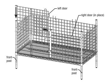
Step 5 - Install top wire shelf (not included) onto top of posts. Rear panel and end panels should lock into top wire shelf.
