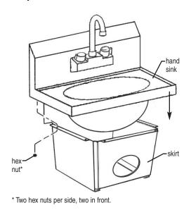
Step 3 - Slide waste receptacle into bottom flanges of skirt.
