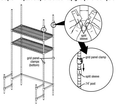
Step 9 - Repeat Step 6 to install remaining wire shelf onto post groove #66.
