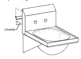
Step 4 - Secure wall brackets to wall.
