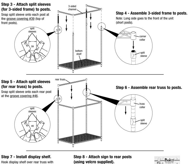
short flange down, allowing front of shelf to rest on 3-sided frame.
