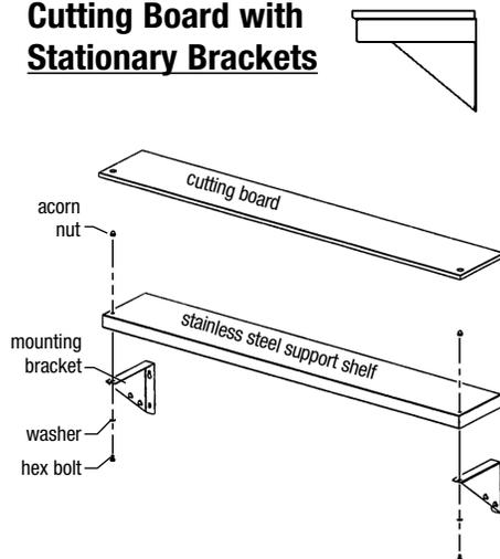
1. Attach mounting brackets to support shelf, using acorn nuts, washers, bolts and predrilled holes. Note: acorn nuts must be at the top.
