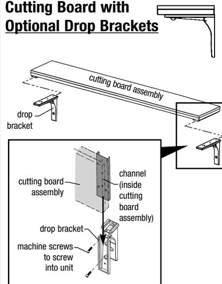
1. Mount drop brackets to table, using machine screws and threaded fasteners on table.
