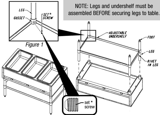
NOTE: Legs and undershaft must be assembled BEFORE securing legs to table.
