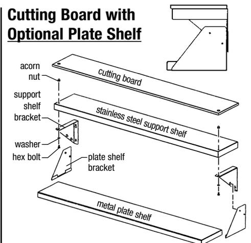
1. Attach shelf support brackets to support shelf, using acorn nuts, washers, bolts and predrilled holes. Note: acorn nuts must be at the top.
