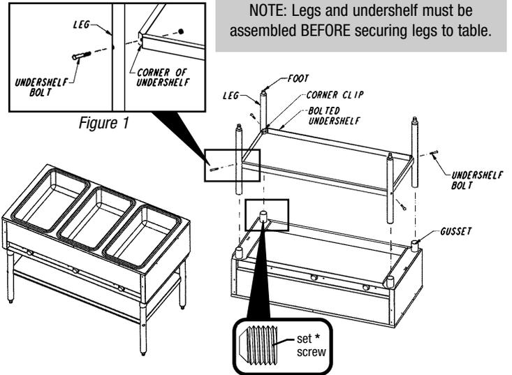
NOTE: Legs and undershaft must be assembled BEFORE securing legs to table.
